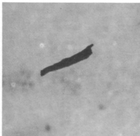
Figure 2 - Polymer remaining after dissolving PHTP with hexane
