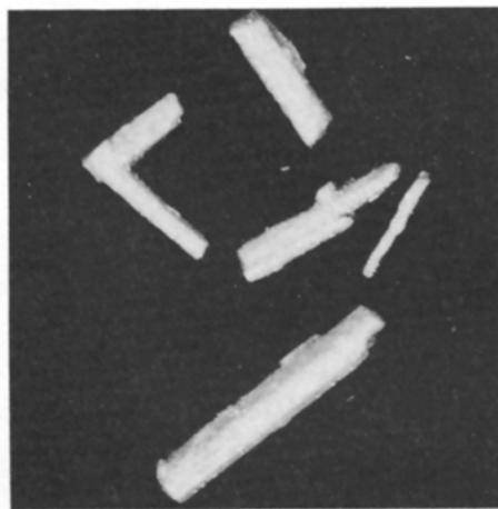
Figure 1A - Polybutadiyne-PHTP Type I single crystals formed by recrystallization out of monomer. 1B - Polybutadiyne-PHTP Type II crystals prepared by diffusion of monomer into host canals.
